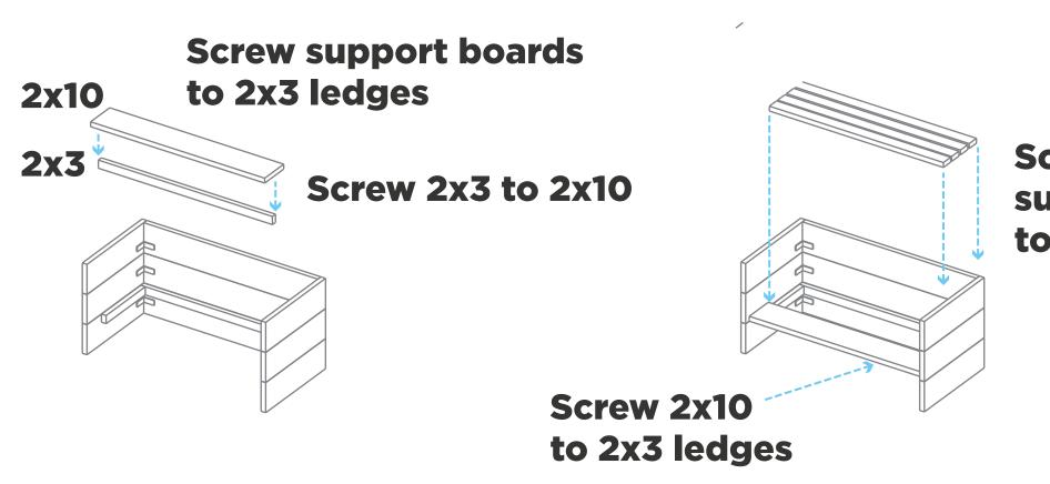
Screw down additional support boards to 2x3 ledges
