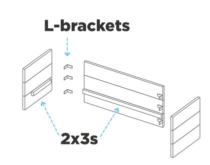
Screw on 2x3 ledges + assemble with L-Brackets
